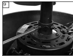
Tighten 2 downrod set screws and lock nuts.
